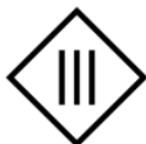
Figure 1 Symbol marking the protection class III (SELV).
