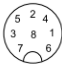
Figure 4 Pin assignment of the connector plug
